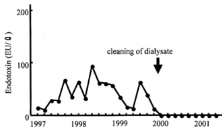
FIG. 2. Ultrapurification of the dialysate and level of endotoxin in the dialysate. In December 1999, the dialysate supply system was completely improved. The level of endotoxin in the dialysate in our hospital before and after the improvement of the system was greatly reduced.
